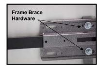
STEP 8 - [Hardware Kit D] Drill 3/8" dia. Hole through frame brace foot, bed, and frame/bed cross member at location shown.
