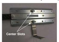
STEP 3 - [Hardware Kit B] Center the assembly against front wall of truck. Select the screw location (A or B) where the silver/grav guide plate fits tightest against the front wall and install self drilling sheet metal screw provided. These screws are used to hold the assembly in place while drilling the mounting holes for the anchor plates. Generally only one screw per side is needed. NOTE: Screws in position A must be removed at a later step while screws in position B may stay in place.
