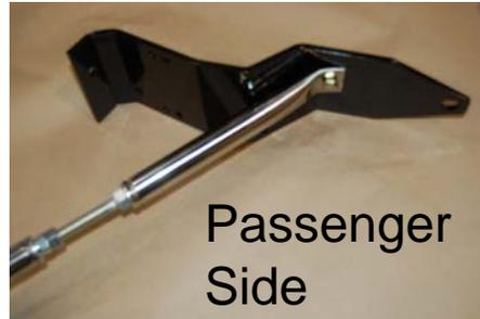
Be sure to connect proper end to bracket. This is the end with the sharper bend and only 1 nut at the end of the threaded rod section. Use the 1/2" long fine thread bolt supplied in the hardware kit..
