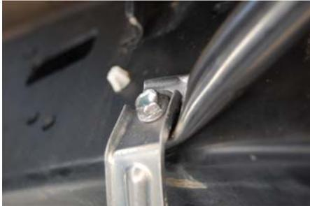
**NOTE:** It may be necessary to loosen the jam nut on the threaded portion of the support brace and lengthen or shorten the brace until the hole in the brace lines up with the hole in the frame.
